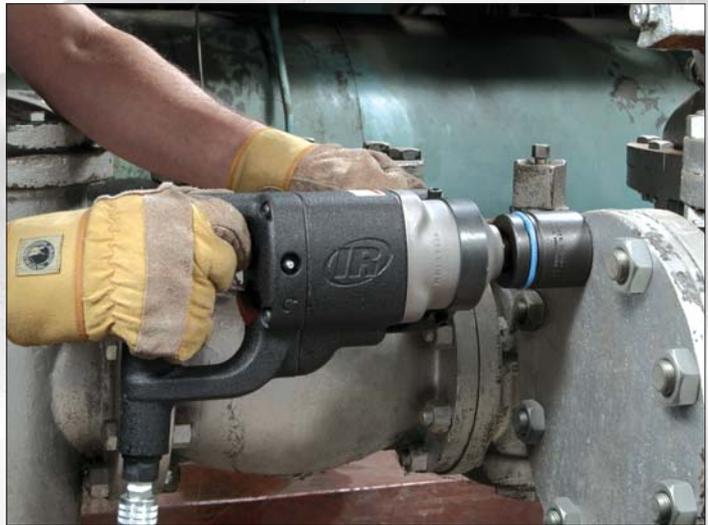
Titanium hammercase provides greater durability with reduced tool weight.
